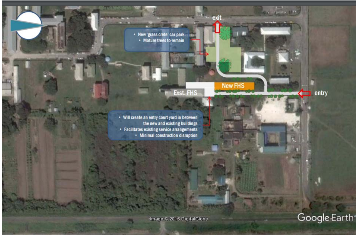
Figure 1 Proposed Site of Building, Road and Car Park (Source: Ian Marfleet)
